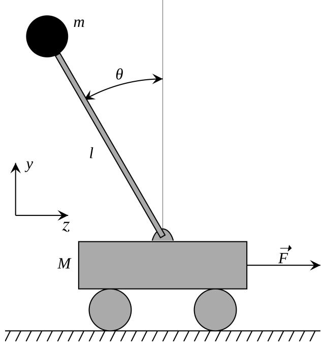
State: position and velocity of the cart, angle and angular velocity of the pole
