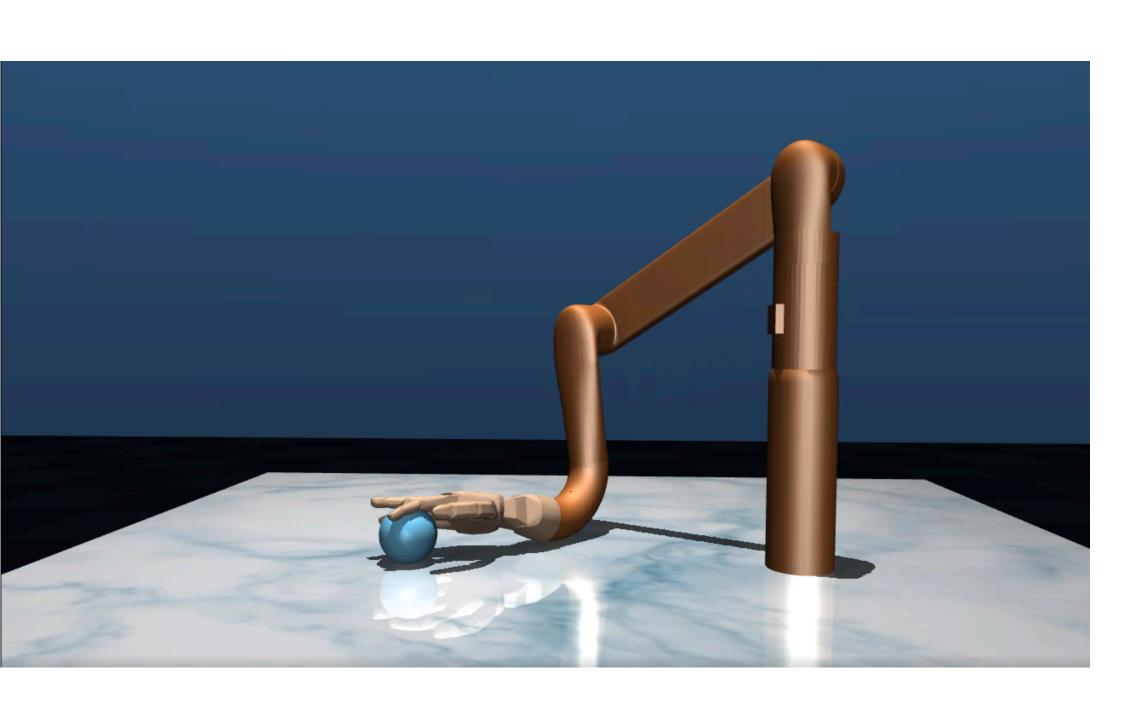
**State** *s*: robot configuration (e.g., joint angles) and the ball's position
