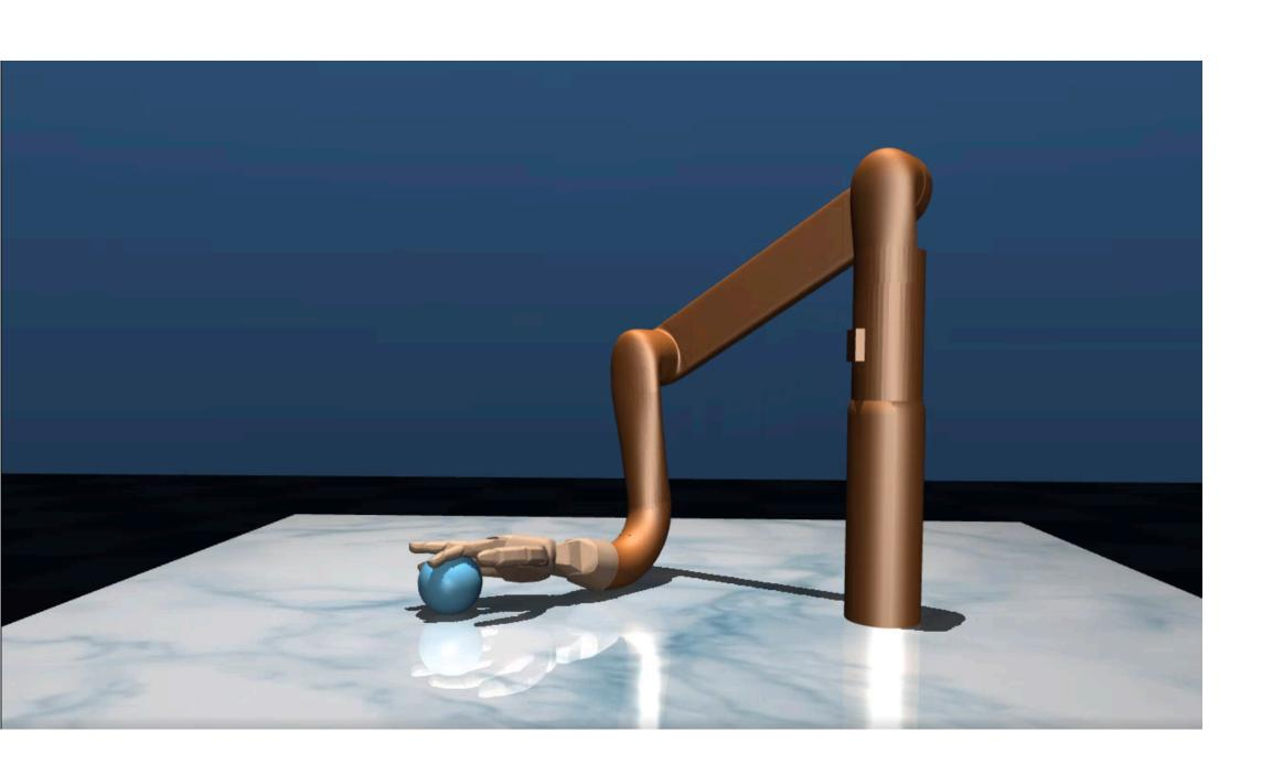
**State** *s*: robot configuration (e.g., joint angles) and the ball's position
